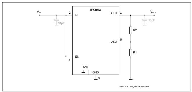
Figure 4 Application Diagram
