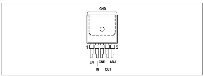
Figure 2 Pin Configuration PG-TO263-5
