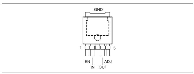
Figure 3 Pin Configuration PG-TO252-5
