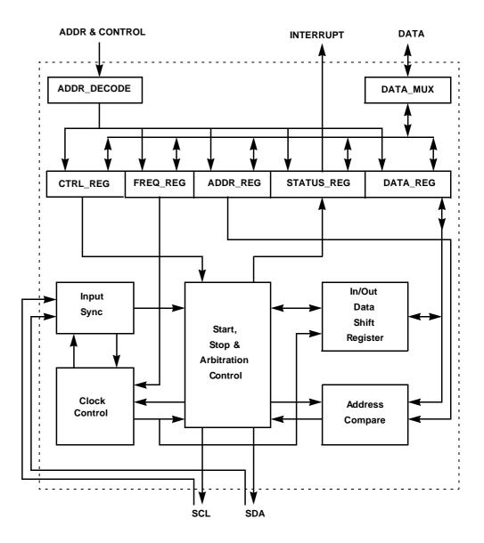
Figure 37 IIC Block Diagram
