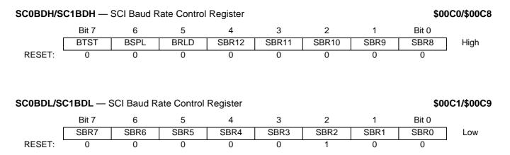
SCxBDH and SCxBDL are considered together as a 16-bit baud rate control register.
