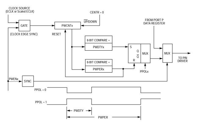
Figure 22 Block Diagram of PWM Left-Aligned Output Channel
