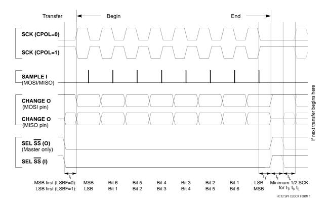
Figure 35 SPI Clock Format 1 (CPHA = 1)
