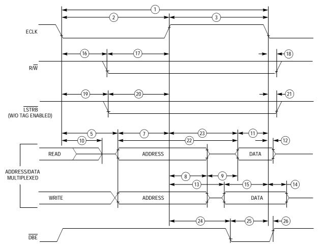
NOTE: Measurement points shown are 20% and 70% of V<sub>DD</sub>
