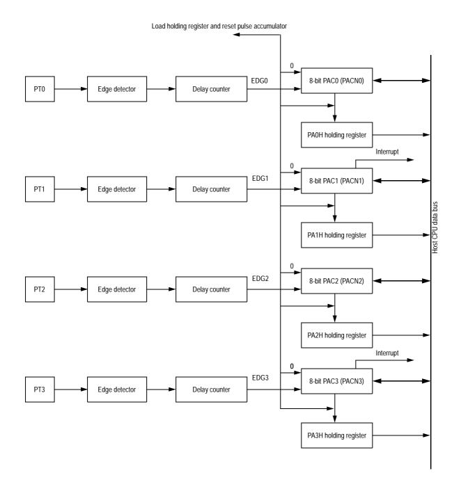
Figure 27 8-Bit Pulse Accumulators Block Diagram
