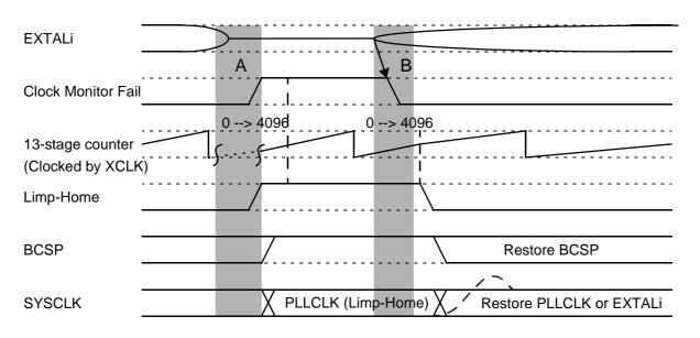
Figure 15 Clock Loss during Normal Operation
