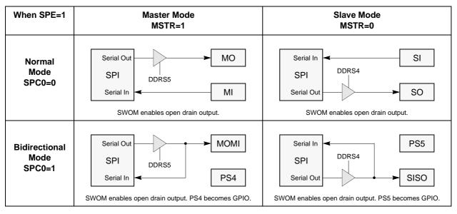
Figure 36 Normal Mode and Bidirectional Mode
