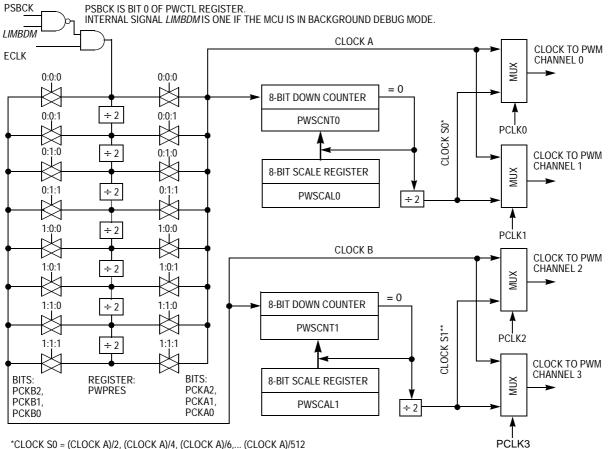
\*CLOCK S0 = (CLOCK A)/2, (CLOCK A)/4, (CLOCK A)/6,... (CLOCK A)/512 \*\*CLOCK S1 = (CLOCK B)/2, (CLOCK B)/4, (CLOCK B)/6,... (CLOCK B)/512
