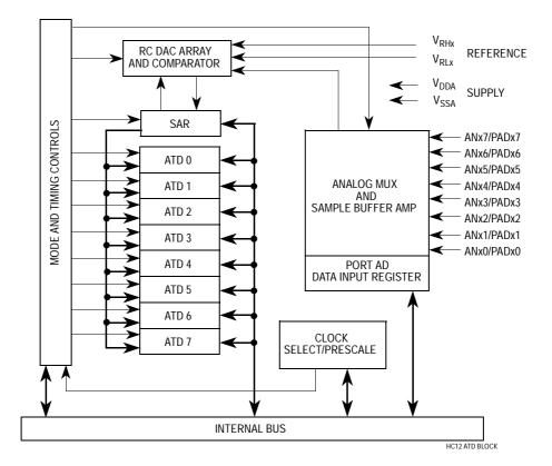
Figure 58 Analog-to-Digital Converter Block Diagram
