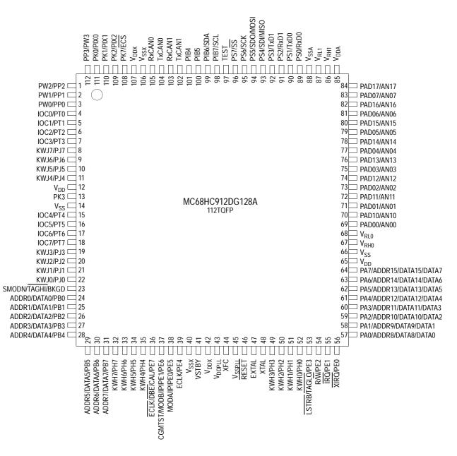
Note: TEST = On early production devices this pin is used for factory test purposes. It is recommended that this pin is not connected within the application, but it may be connected to VSS or 5.5V max without issue. On later production devices this pin is not bonded out.
