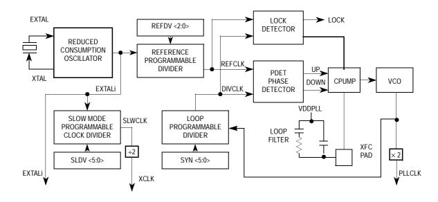
Figure 14 PLL Functional Diagram
