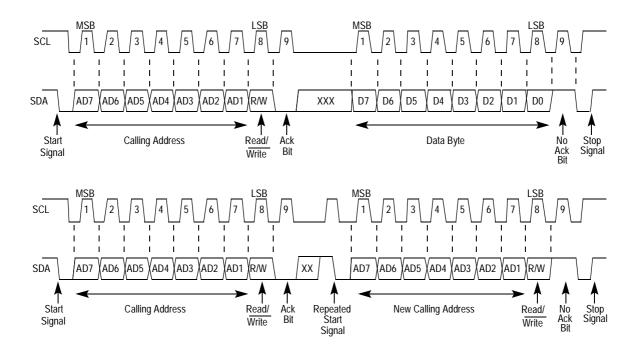
Figure 38 IIC Transmission Signals
