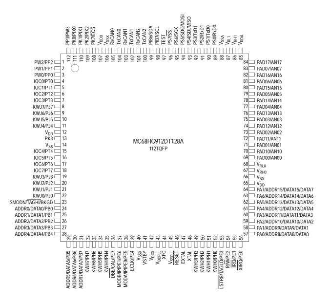
Note: TEST = On early production devices this pin is used for factory test purposes. It is recommended that this pin is not connected within the application, but it may be connected to VSS or 5.5V max without issue. On later production devices this pin is not bonded out.
