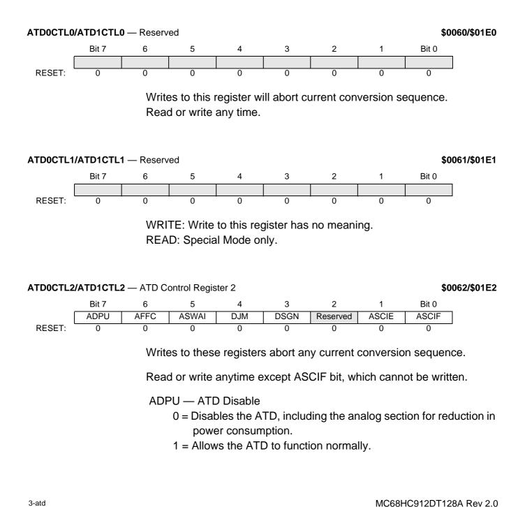
Software can disable the clock signal to the A/D converter and power down the analog circuits to reduce power consumption. When reset to zero, the ADPU bit aborts any conversion sequence in progress. Because the bias currents to the analog circuits are turned off, the ATD requires a period of recovery time to stabilize the analog circuits after setting the ADPU bit.
