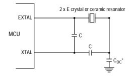
Due to the nature of the translated ground Colpitts oscillator a DC voltage bias is applied to the crystal.
