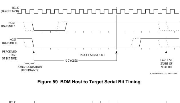
speed up rising edges. Since the target does not drive the BKGD pin during this period, there is no need to treat the line as an open-drain signal during host-to-target transmissions.
