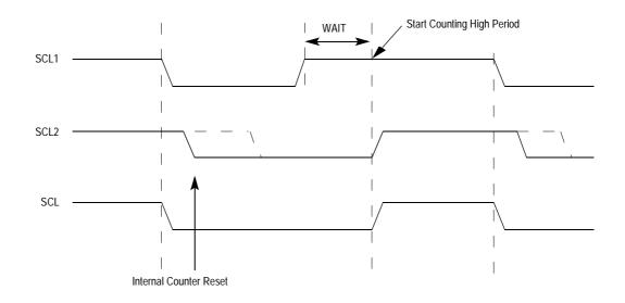
Figure 39 IIC Clock Synchronization
