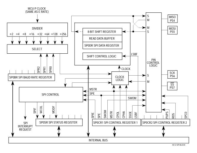
Figure 33 Serial Peripheral Interface Block Diagram
