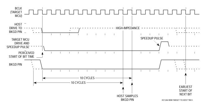
Figure 61 BDM Target to Host Serial Bit Timing (Logic 0)
