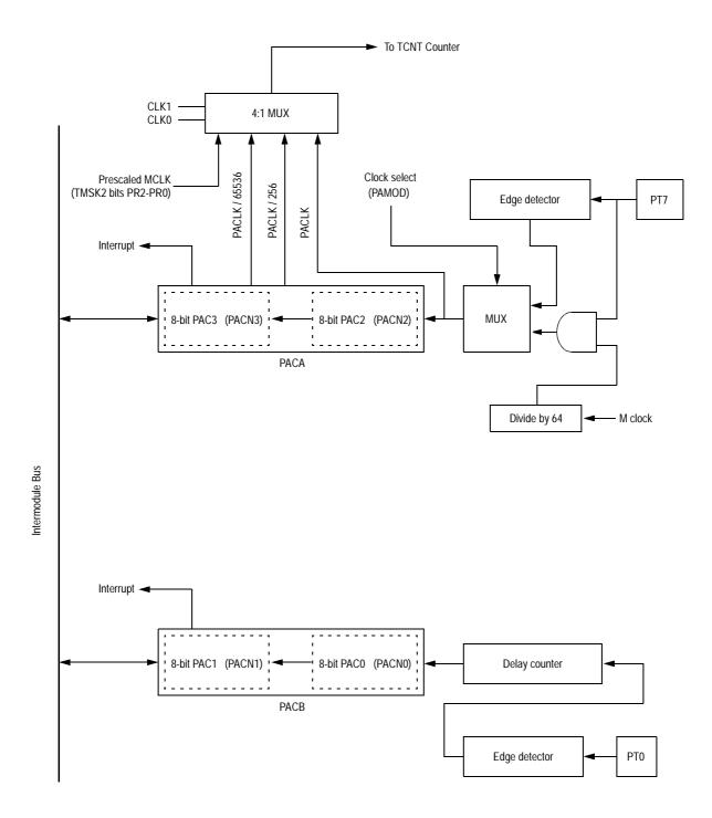
Figure 28 16-Bit Pulse Accumulators Block Diagram
