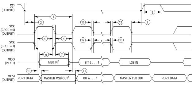
1.  $\overline{SS}$  output mode (DDS7 = 1, SSOE = 1). 2. LSBF = 0. For LSBF = 1, bit order is LSB, bit 1, ..., bit 6, MSB.
