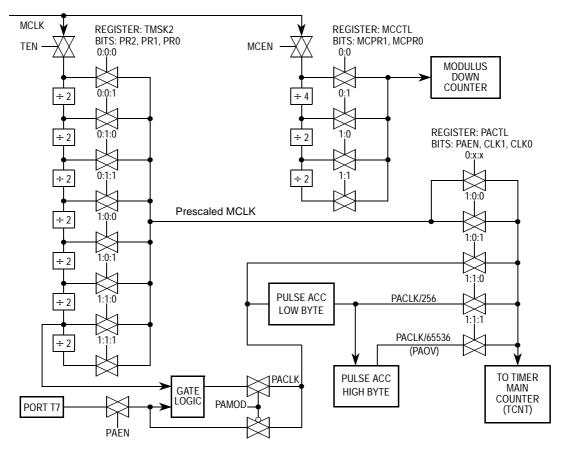
Figure 20 Clock Chain for ECT
