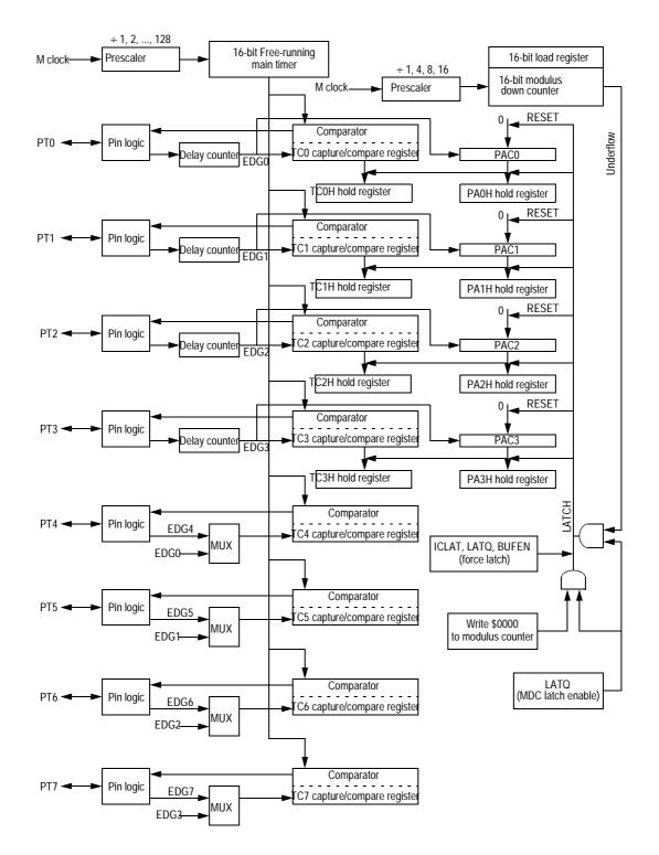
Figure 25 Timer Block Diagram in Latch Mode
