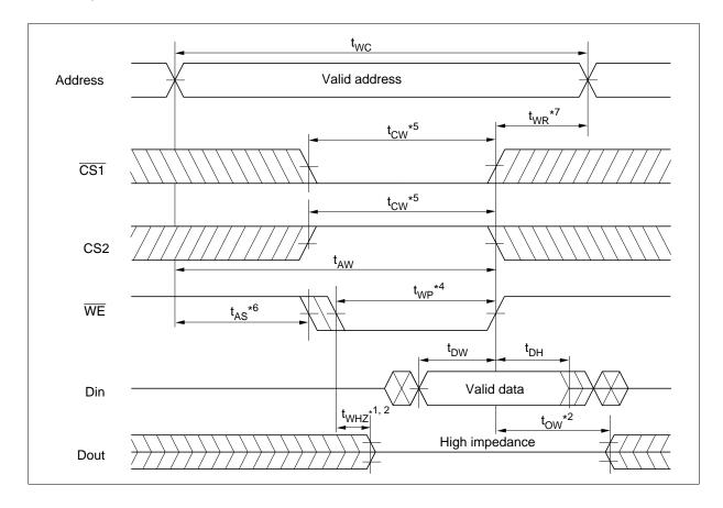
Write Cycle (2) ( $\overline{\text{CS}}$  Clock,  $\overline{\text{OE}} = V_{\text{IH}}$ )
