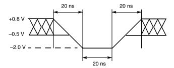
Figure 12.2 Maximum Positive Overshoot Waveform
