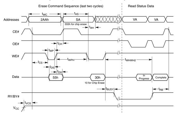
Figure 17.7 Chip/Sector Erase Operation Timings
