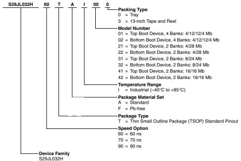
3.0 Volt-only, 32 Megabit (2 M x 16-Bit/4 M x 8-Bit) Simultaneous Read/Write Flash Memory Manufactured on 130 nm process technology
