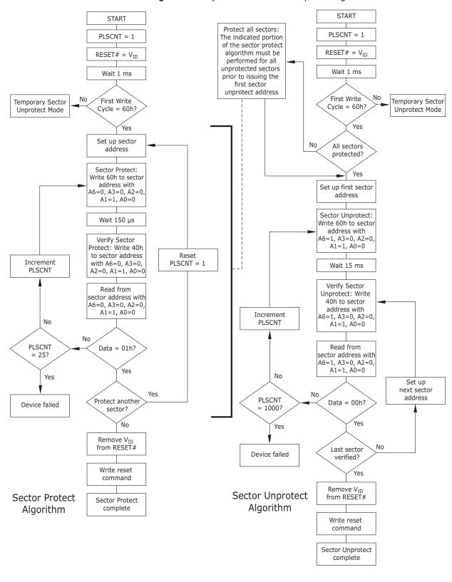
Figure 8.2 In-System Sector Protect/Unprotect Algorithms
