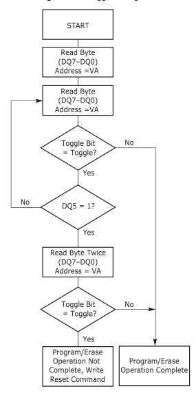
Figure 11.2 Toggle Bit Algorithm
