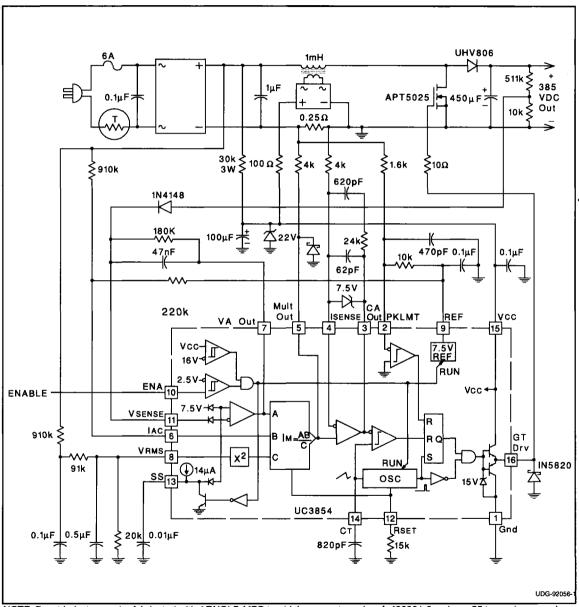
NOTE: Boost inductor can be fabricated with ARNOLD MPP toroidal core part number A-438381-2, using a 55 turn primary and a 13 turn secondary.
