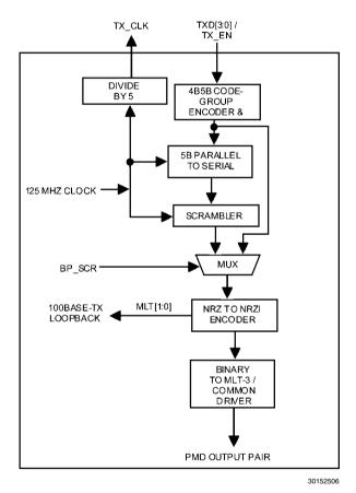
FIGURE 5. 100BASE-TX Transmit Block Diagram
