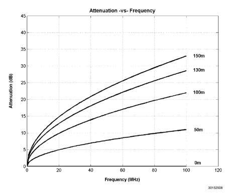
FIGURE 7. EIA/TIA Attenuation vs. Frequency for 0, 50, 100, 130 & 150 Meters of CAT 5 Cable
