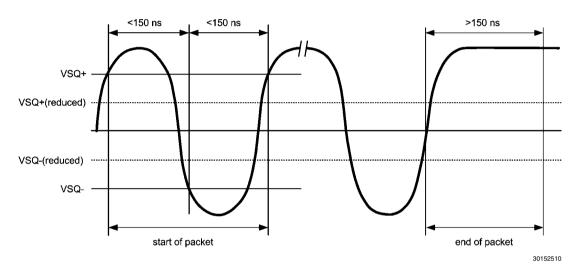
FIGURE 9. 10BASE-T Twisted Pair Smart Squelch Operation
