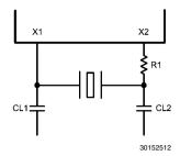
**FIGURE 11. Crystal Oscillator Circuit**
