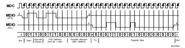
FIGURE 3. Typical MDC/MDIO Read Operation
