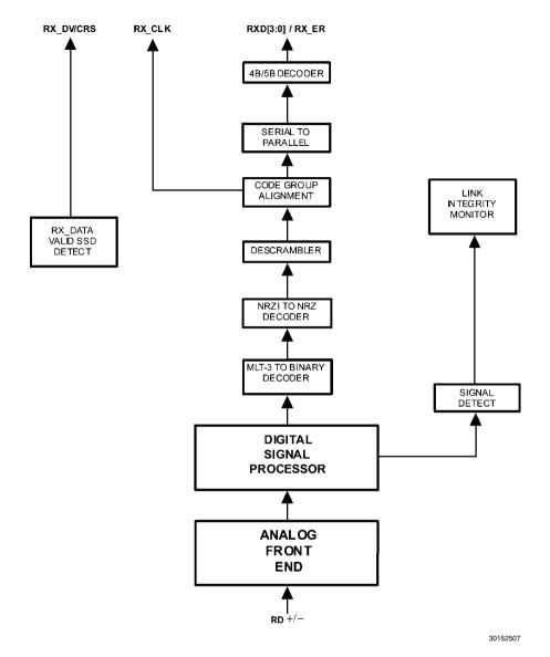
FIGURE 6. 100BASE-TX Receive Block Diagram
