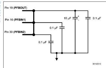
FIGURE 12. Power Feedback Connection
