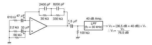
Fig. 3 Flat Noize Measurement Circuit (FLAT + JIS A)
