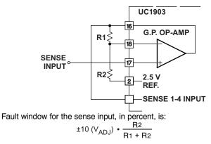
A. The general purpose op-amp on the UC1903 can be used to create a sense input with an independently tighter fault window.
