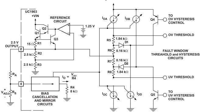
A. The UC1903 fault window circuitry generates OV and UV thresholds centered around the 2.5-V reference. Window magnitude and threshold hysteresis are proportional to the window adjust input voltage at Pin 4.
