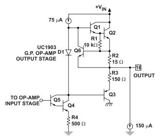
A. The G.P. op-amp on the UC1903 has a high source current (20 mA) capability and enhanced transient sinking capability through substrate device Q3.
