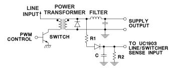
Figure 7. Line/Switcher Sense Input Used for Early Line or Switcher Fault Indication
