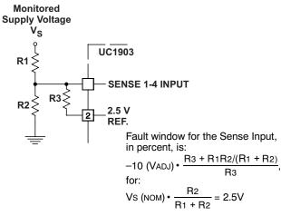
A. Using the reference output and a resistive divider, a sense input with an independently wider fault window can be generated.
