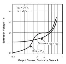
Figure 4. UC1525A Output Saturation Characteristics.
