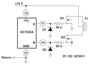
Figure 3. Output Drivers With Low Source Impedance
