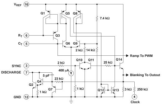
Figure 7. UC1525A Oscillator Schematic
