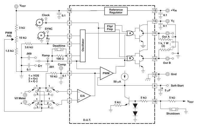
Figure 12. Lab Test Fixture
