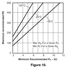
Oscillator Discharge Time vs  $R_T\,C_T$
