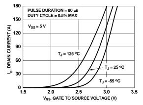
Figure 5. Transfer Characteristics
