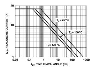
Figure 9. Unclamped Inductive Switching Capability
