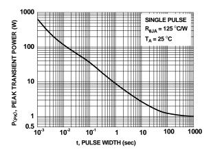
Figure 12. Single Pulse Maximum Power Dissipation
