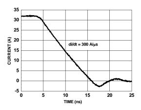
Figure 14. FDMS7558S SyncFET body diode reverse recovery characteristic
