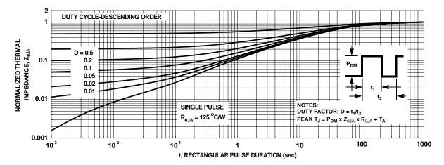
Figure 13. Junction-to-Ambient Transient Thermal Response Curve
