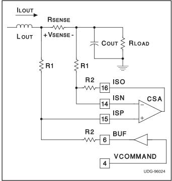
Figure 5. Configuring the Current Sense Amplifier
