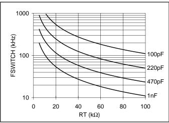
Figure 3. Programming Switching Frequency with CT
