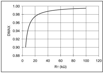
Figure 2. Programming Maximum Duty Cycle with RT
