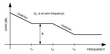
Figure 30. Output-Control Transfer Function
