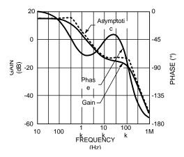
Figure 29. Control-Output Transfer Function
