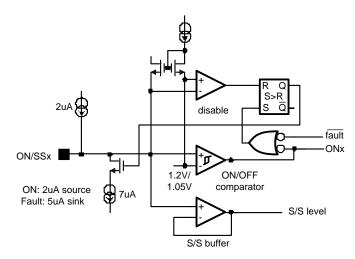
Figure 22. Soft Start and ON/OFF
