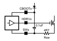
Figure 25. SW Series Resistor
