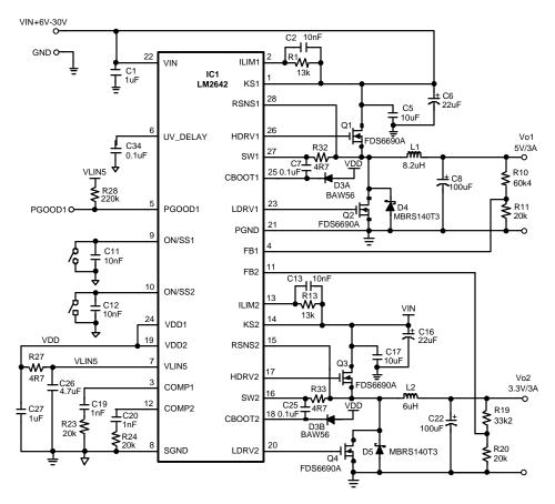
Figure 2. Typical 2 Channel Application Circuit
