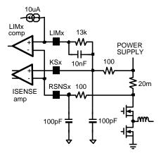
Figure 26. Current Sense and Current Limit
