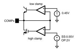
Figure 23. Voltage Clamp at COMPx Pin
