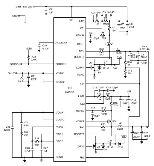
Figure 3. Typical Single Channel Application Circuit
