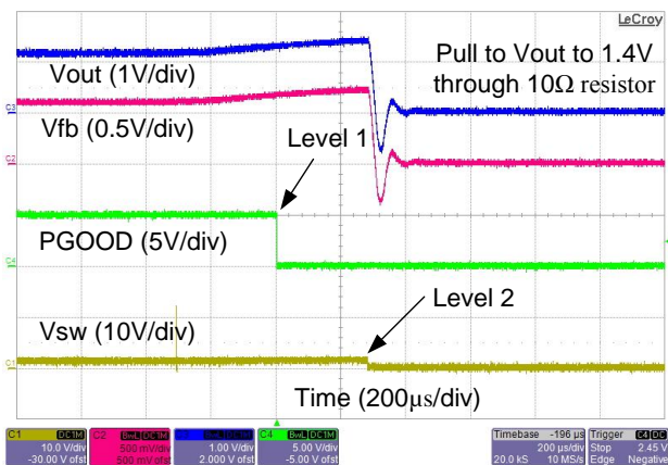
Figure 23. Over-Voltage Protection Level 1 and Level 2
