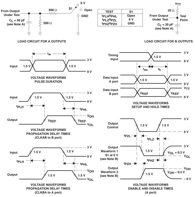
NOTES: A. C<sub>L</sub> includes probe and jig capacitance.
