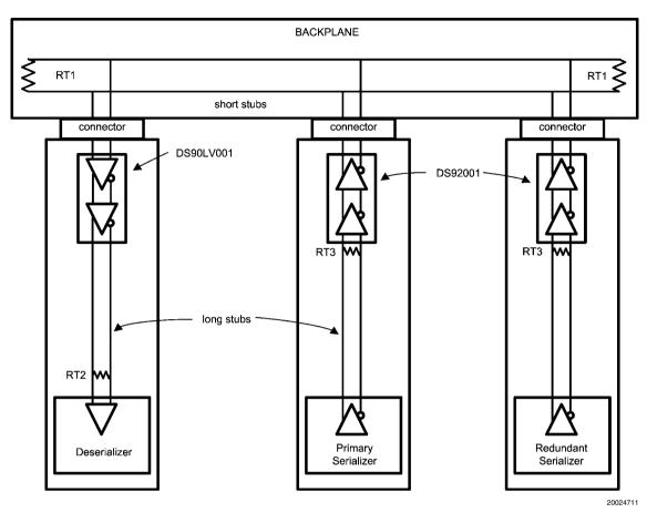
FIGURE 8. Backplane Stub-Hider Application
