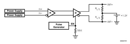
FIGURE 6. TRI-STATE Delay Test Circuit
