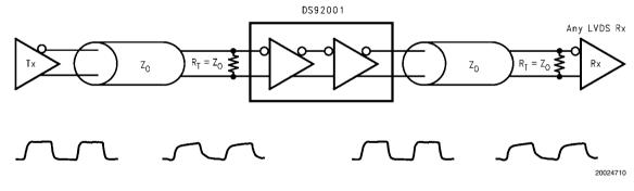
FIGURE 9. Cable Repeater Application
