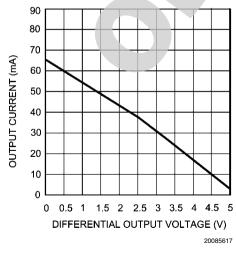
Output Current vs. Receiver Output High Voltage
