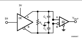
FIGURE 5. Test Circuit for Receiver Propagation Delay
