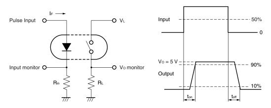
\*2 The turn-on time and turn-off time are specified as input-pulse width ≥ 0.5 ms.
