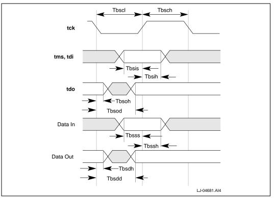
Figure 10-4. Boundary-Scan Tristate Timing
