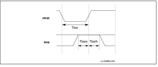
Table 10-2 shows the SA-110 boundary-scan interface timing specifications.
