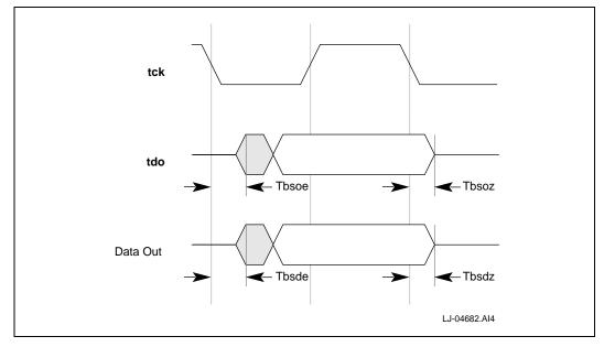
Figure 10-5. Boundary-Scan Reset Timing
