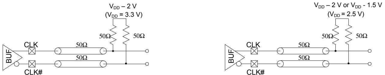
Figure 8. LVPECL Termination
