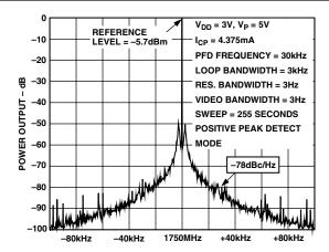
TPC 10. ADF4218 RF Reference Spurs (1750 MHz, 30 kHz, 3 kHz)
