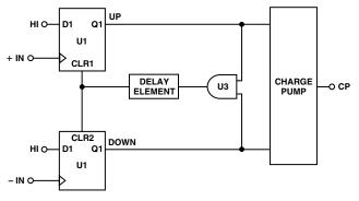
Figure 5. PFD Simplified Schematic
