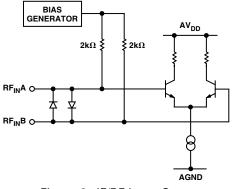
Figure 3. IF/RF Input Stage
