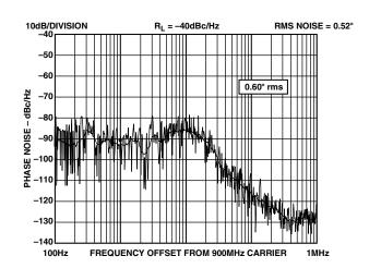
TPC 16. ADF4218 IF Integrated Phase Noise (540 MHz, 200 kHz, 20 kHz)
