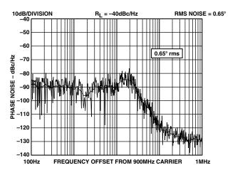
TPC 6. ADF4218 RF Integrated Phase Noise (900 MHz, 200 kHz, 35 kHz)
