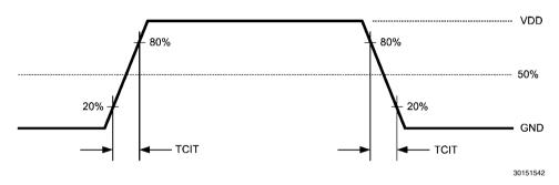
FIGURE 5. DS90C185 (Transmitter) Input Clock Transition Time
