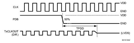
FIGURE 9. Transmitter Power Down Delay
