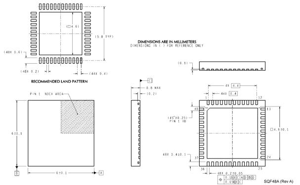
48-Lead LLP Quad Package Dimensions in millimeters only TI Package Number SQF48A
