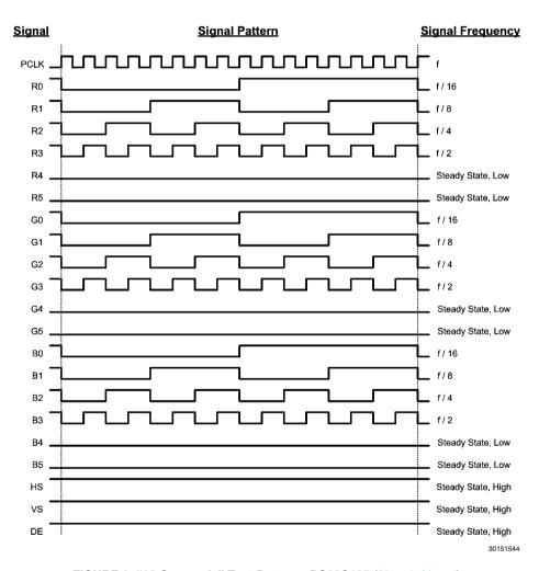
FIGURE 2. "16 Grayscale" Test Pattern - DS90C185 (Note 8, Note 9)
