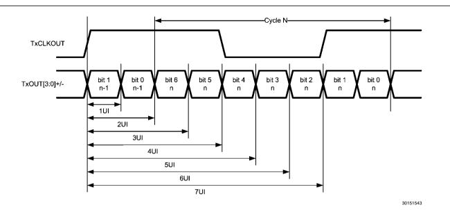
FIGURE 10. Transmitter LVDS Output Pulse Position Measurement - DS90C185
