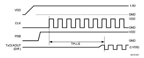
FIGURE 8. DS90C185 (Transmitter) Phase Lock Loop Set Time
