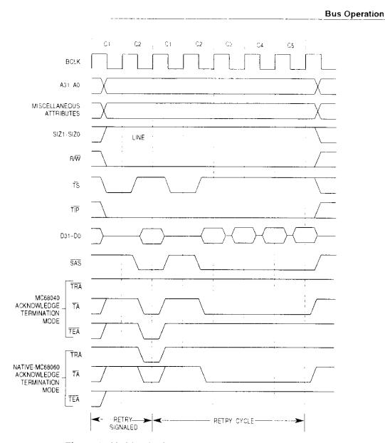
Figure 7-40. Line Write Retry Bus Cycle Timing
