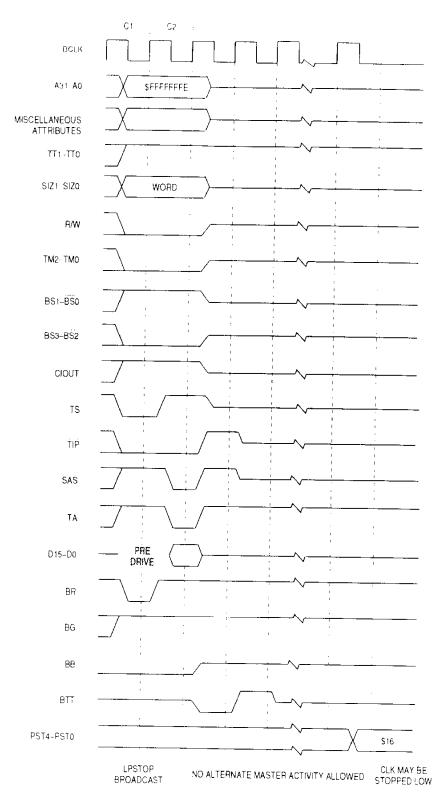
Figure 7-33. LPSTOP Broadcast Bus Cycle Timing,  $\overline{\text{BG}}$  Negated
