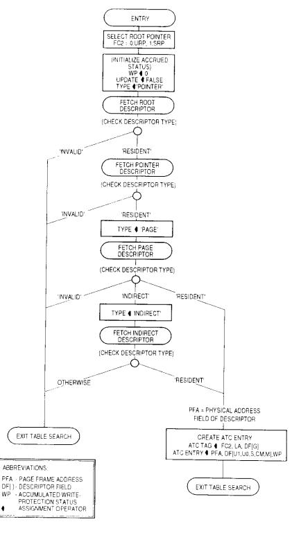
Figure 4-8. Detailed Flowchart of Table Search Operation
