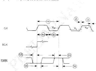
Figure 12-12. Clock Input Timing Diagram
