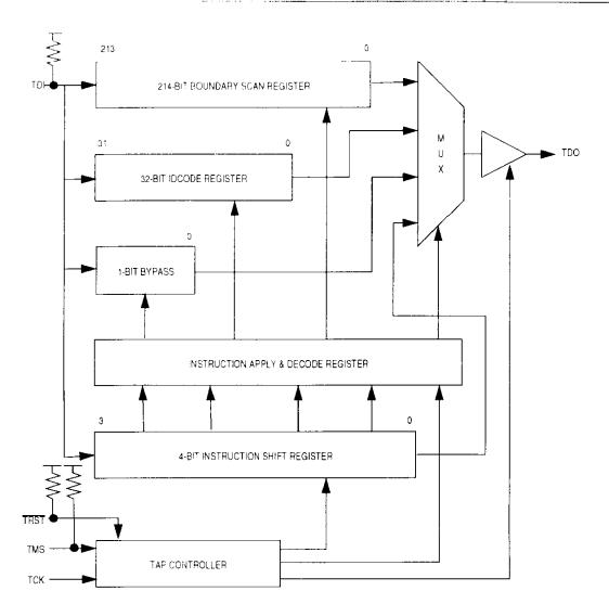
Figure 9-1. JTAG Test Logic Block Diagram
