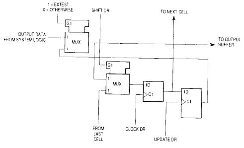
Figure 9-3. Output Pin Cell (O.Pin)
