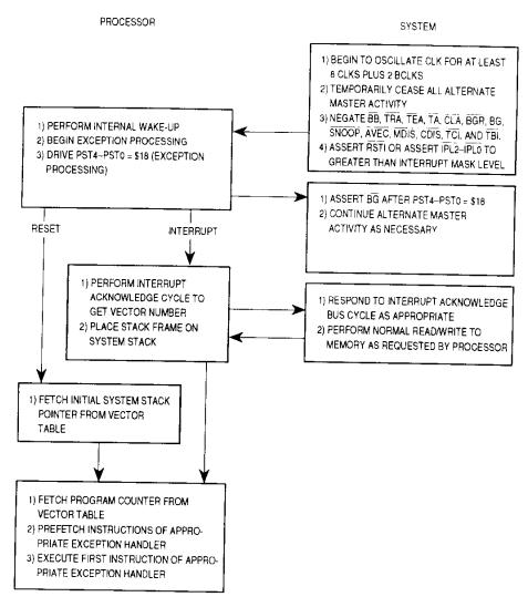
Figure 7-35. Exiting LPSTOP Mode Flowchart
