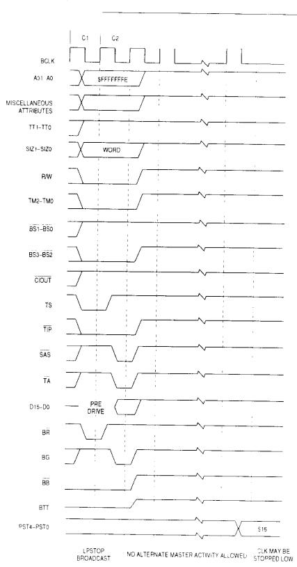
Figure 7-34. LPSTOP Broadcast Bus Cycle Timing,  $\overline{\text{BG}}$  Asserted
