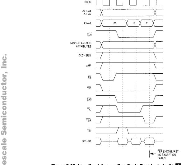
Figure 7-38. Line Read Access Bus Cycle Terminated with TEA Timing
