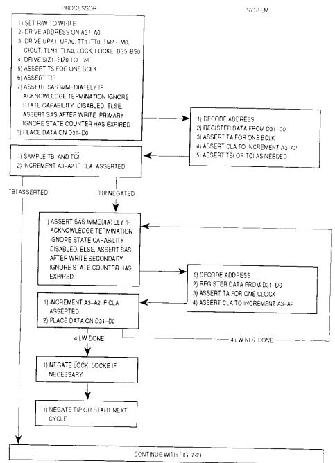
Figure 7-20. Line Write Cycle Flowchart
