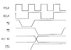
Figure 11-5. MC68040 Address Hold Time
