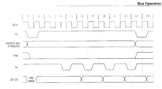
Figure 7-52. Extra Data Write Hold Example
