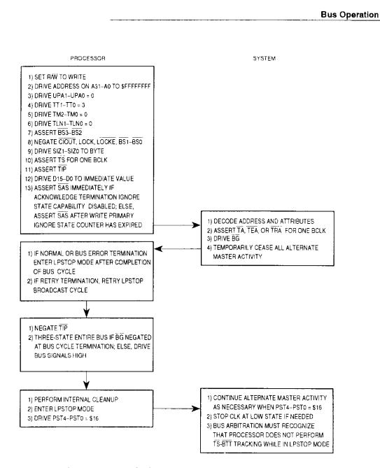
Figure 7-32. LPSTOP Broadcast Cycle Flowchart
