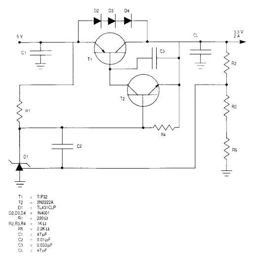
Figure 11-1. Linear Voltage Regulator Solution
