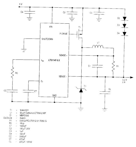
Figure 11-2. LTC1147 Voltage Regulator Solution
