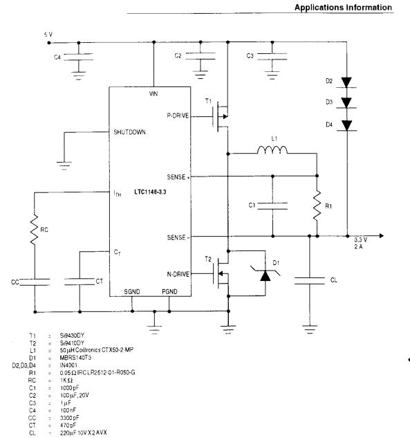
Figure 11-3. LTC1148 Voltage Regulator Solution
