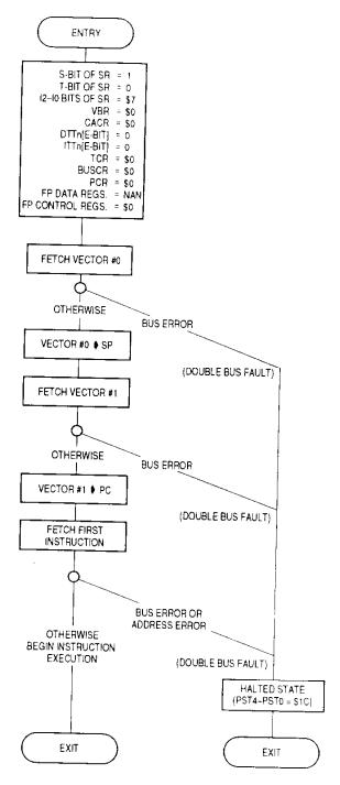
Figure 8-5. Reset Exception Processing Flowchart
