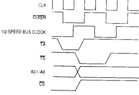
Figure 11-6. MC68060 Address Hold Time
