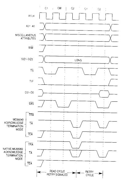
Figure 7-39. Retry Read Bus Cycle Timing
