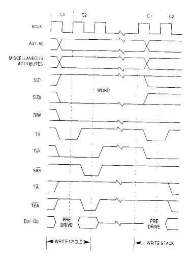
Figure 7-37. Word Write Access Bus Cycle Terminated with TEA Timing
