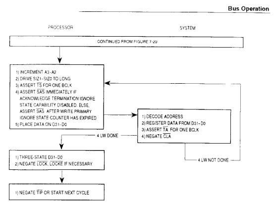
Figure 7-21. Line Write Burst-Inhibited Cycle Flowchart
