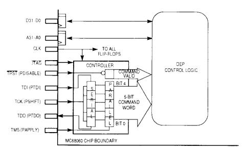
Figure 9-10. Debug Command Interface Schematic
