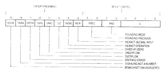
Figure 6-3. Floating-Point Control Register Format
