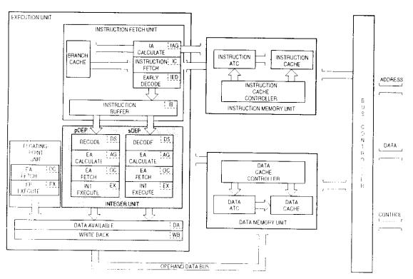
Figure 3-1. MC68060 Integer Unit Pipeline
