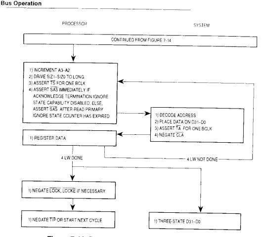
Figure 7-16. Burst-Inhibited Line Read Cycle Flowchart
