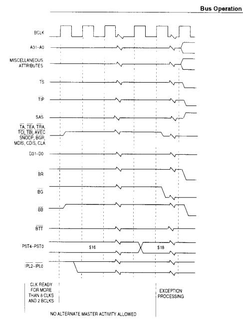
Figure 7-36. Exiting LPSTOP Mode Timing Diagram
