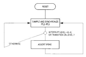
Figure 7-25. Interrupt Pending Procedure
