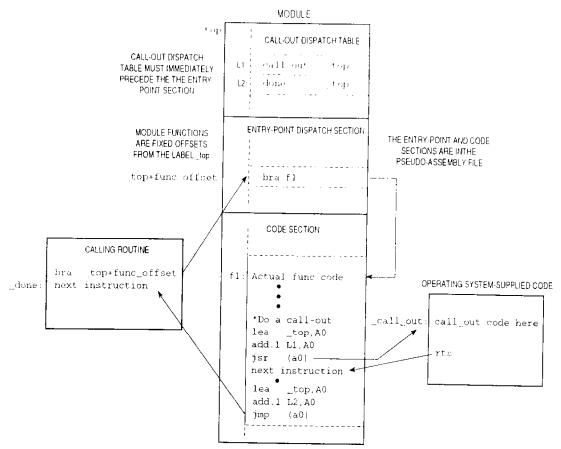
Figure C-3. Module Call-In, Call-Out Example
