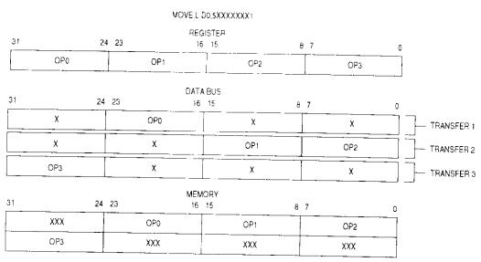
Figure 7-9. Example of a Misaligned Long-Word Transfer
