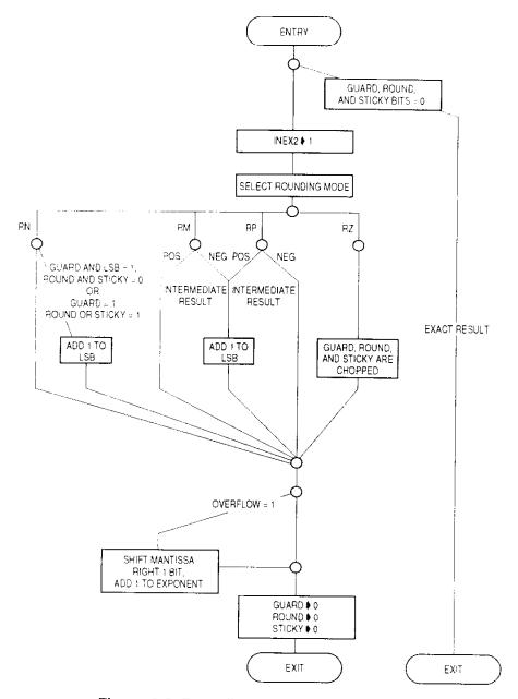
Figure 6-9. Rounding Algorithm Flowchart
