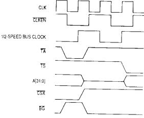
Figure 11-7. MC68060 Address Hold Time Fix
