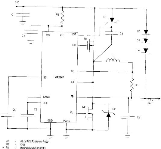
Motorola MMDF3N03HD Central Semi, CMPSM-3 D1 Motorola MBRS 120T3 2x 47µF, 20V AVXTPSD476K020R D2 C1 C2
