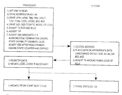
Figure 7-12. Byte, Word, and Long-Word Read Cycle Flowchart
