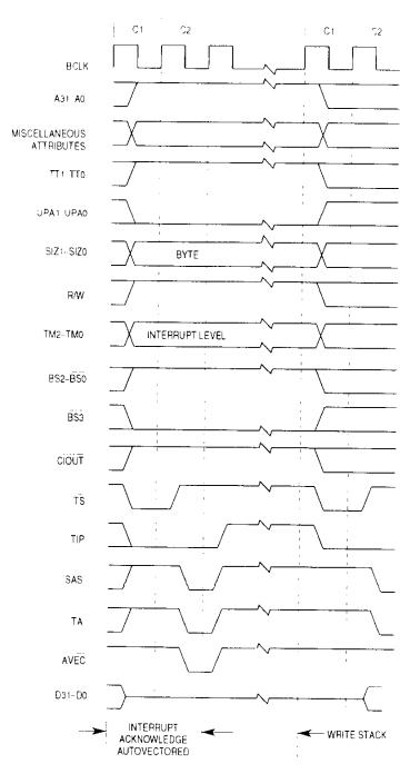
Figure 7-29. Autovector Interrupt Acknowledge Bus Cycle Timing
