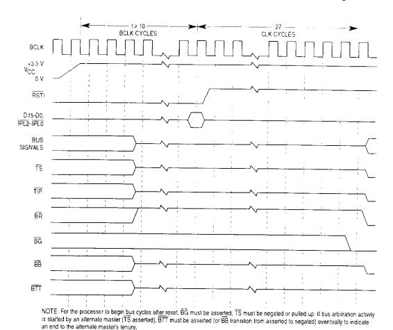
Figure 7-48. Initial Power-On Reset Timing
