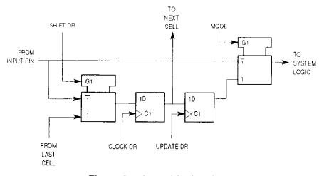
Figure 9-5. Input Pin Cell (I.Pin)
