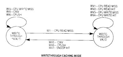
Figure 5-7. Data Cache Line State Diagrams
