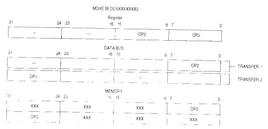
Figure 7-10. Example of Misaligned Word Transfer
