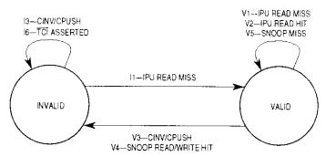
Figure 5-6. Instruction Cache Line State Diagram
