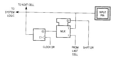
Figure 9-4. Observe-Only Input Pin Cell (I.Obs)
