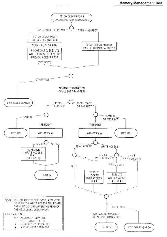
Figure 4-9. Detailed Flowchart of Descriptor Fetch Operation
