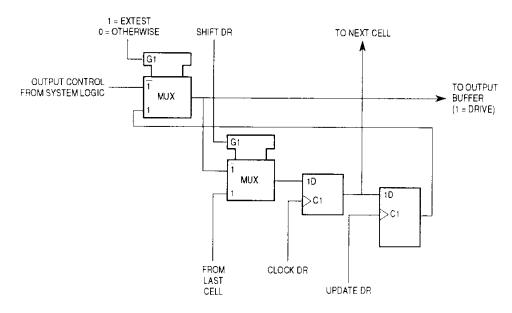
Figure 9-6. Output Control Cell (IO.Ctl)
