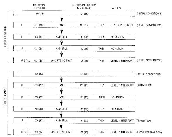
Figure 8-3. Interrupt Recognition Examples
