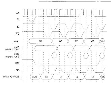
Figure 7-24. Using CLA in a High-Speed DRAM Design
