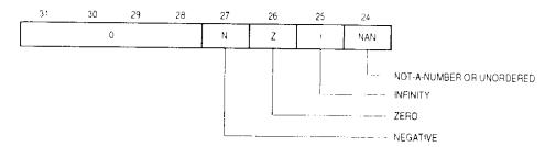
Figure 6-4. Floating-Point Condition Code (FPSR)
