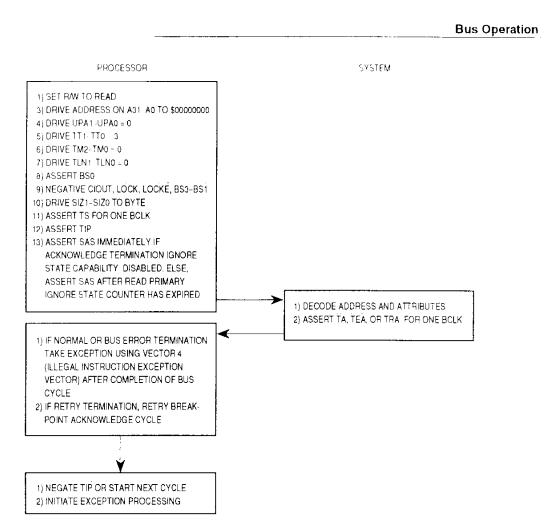
Figure 7-30. Breakpoint Interrupt Acknowledge Cycle Flowchart
