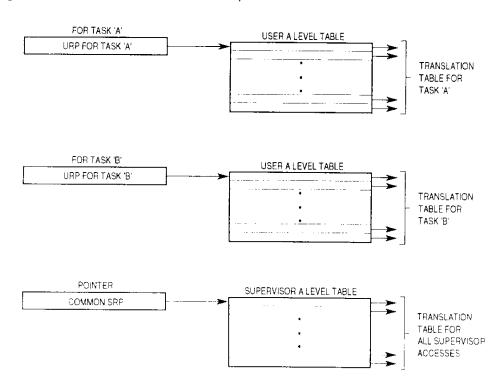
Figure 4-16. Translation Table Structure for Two Tasks
