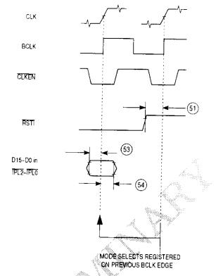
Figure 12-14. Reset Configuration Timing
