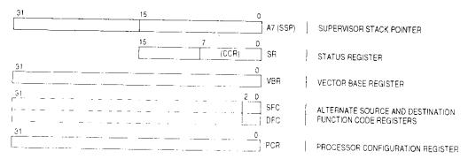
Figure 3-3. Integer Unit Supervisor Programming Model
