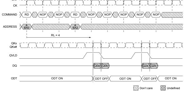
Remark RD : READ command A/BAp: Address A of bank p RL : READ latency Qpq : Data q from bank p
