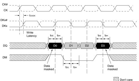
Figure 2-7. Basic WRITE Burst / DM Timing
