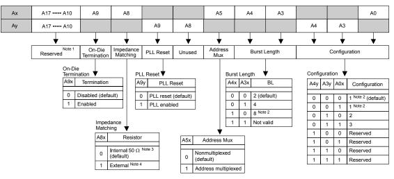
Figure 2-27. Mode Register Set Command in Multiplexed Address Mode
