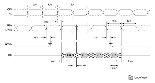
Figure 2-13. Basic READ Burst Timing
