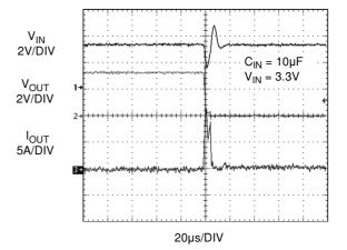
Figure 18. Short Circuit Response Time (Output shorted to ground)
