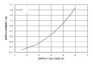
Figure 2. Quiescent Current vs. Input Voltage
