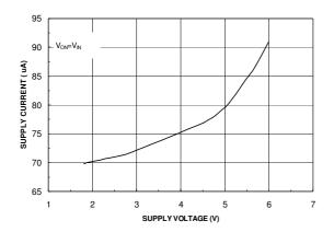
Figure 1. Quiescent Current vs. Input Voltage
