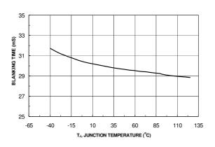
Figure 15.  $T_{BLANK}$  vs. Temperature
