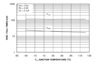
Figure 13.  $T_{\mbox{\scriptsize RISE}}\,/\,T_{\mbox{\scriptsize FALL}}$  vs. Temperature
