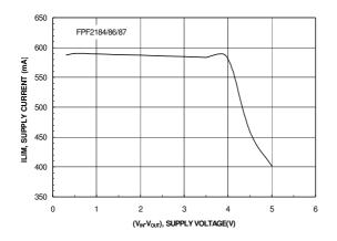
Figure 7. Current Limit vs. Output Voltage
