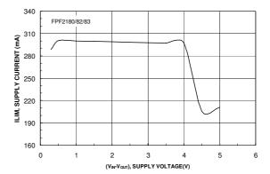
Figure 6. Current Limit vs. Output Voltage
