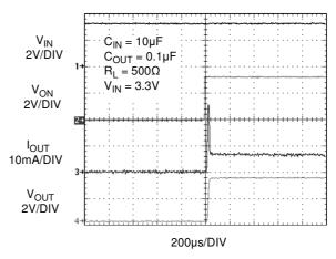
Figure 16. T<sub>ON</sub> Response
