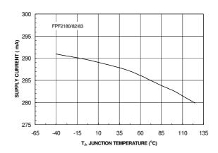
Figure 8. Current Limit vs. Temperature
