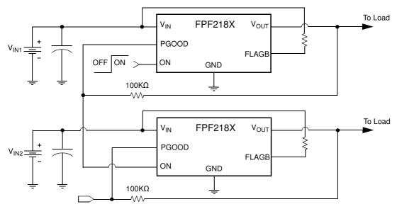
Power good function in sequential startup. No battery is loaded to the output
