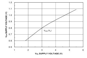
Figure 5.  $V_{ON}$  Low Voltage vs. Input Voltage
