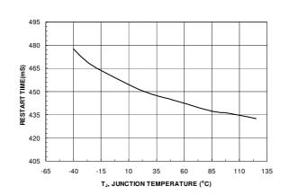
Figure 14. T<sub>RESTART</sub> vs. Temperature
