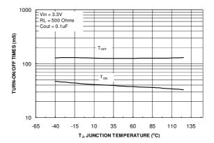
Figure 12.  $T_{ON}$  /  $T_{OFF}$  vs. Temperature
