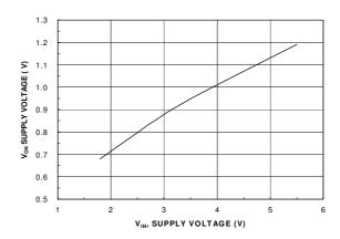
Figure 4.  $V_{ON}$  High Voltage vs. Input Voltage
