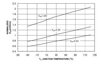
Figure 11.  $R_{ON}$  vs. Temperature
