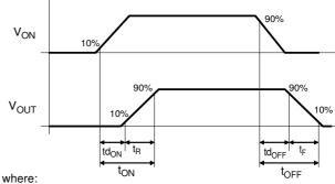
$\begin{array}{l} td_{ON} = Delay \ On \ Time \\ t_R = V_{OUT} \ Rise \ Time \\ t_{ON} = Turn \ On \ Time \\ td_{OFF} = Delay \ Off \ Time \\ t_F = V_{OUT} \ Fall \ Time \\ t_{OFF} = Turn \ Off \ Time \end{array}$
