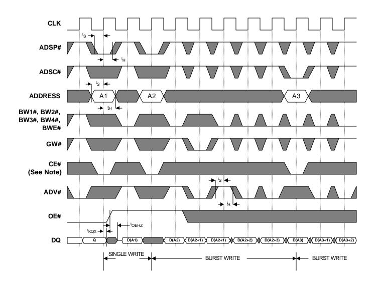
Note: CE# active in this timing diagram means that all chip enables CE#, CE2, and CE2# are active.
