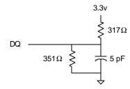
Fig. 2 OUTPUT LOAD EQUIVALENT
