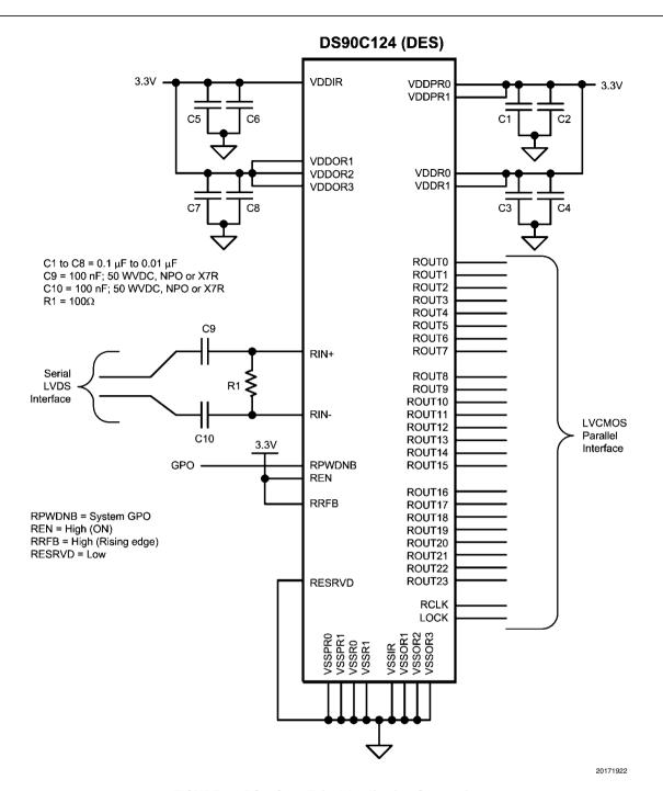
FIGURE 19. DS90C124 Tyical Application Connection
