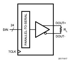
$\label{eq:VOD} VOD = (D_{OUT+}) - (D_{OUT-})$  Differential output signal is shown as  $(D_{OUT+}) - (D_{OUT-})$ , device in Data Transfer mode.
