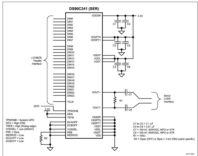
FIGURE 18. DS90C241 Tyical Application Connection
