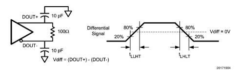
FIGURE 3. Serializer LVDS Output Load and Transition Times
