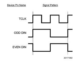
FIGURE 1. Serializer Input Checker-board Pattern
