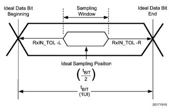
RxIN\_TOL\_L is the ideal noise margin on the left of the figure, with respect to ideal. RxIN\_TOL\_R is the ideal noise margin on the right of the figure, with respect to ideal.
