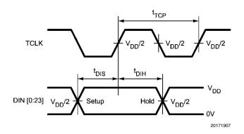
FIGURE 5. Serializer Setup/Hold Times
