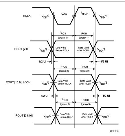
FIGURE 15. Deserializer Setup and Hold Times
