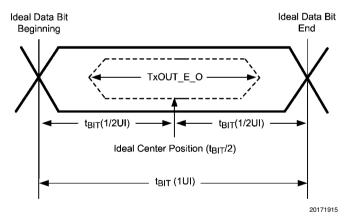
FIGURE 9. Transmitter Output Eye Opening (TxOUT\_E\_O)
