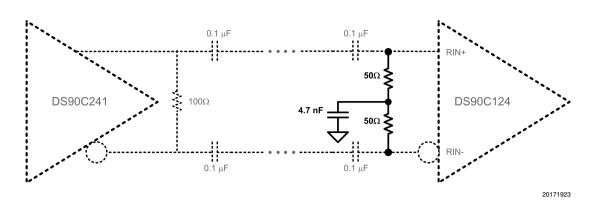
FIGURE 20. Receiver Termination Option 2
