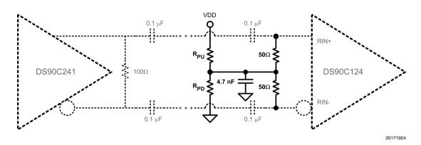
FIGURE 21. Receiver Termination Option 3
