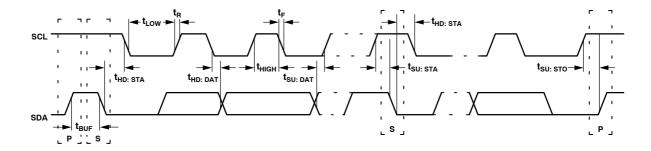
Figure 2. Serial Bus Timing Diagram
