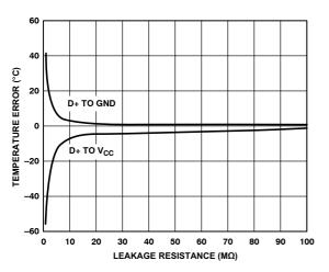
Figure 3. Remote Temperature Error vs. PCB Resistance
