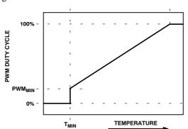
Figure 53. PWM<sub>MIN</sub> Determines Minimum PWM Duty Cycle
