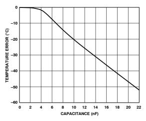
Figure 4. Temperature Error vs. Capacitance
