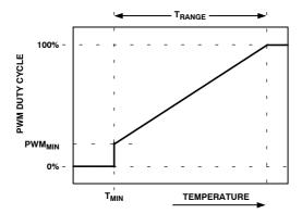
Figure 56. T<sub>RANGE</sub> Parameter Affects Cooling Slope
