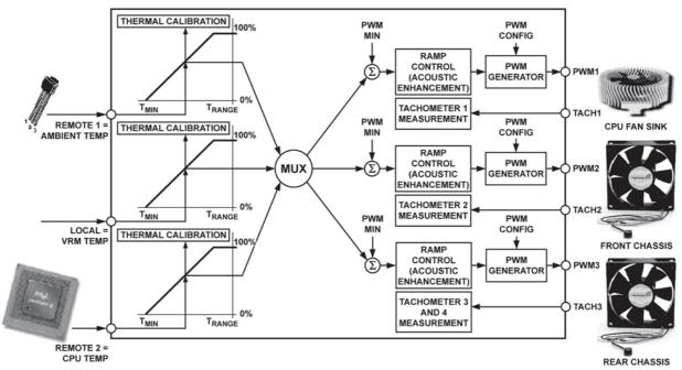
Figure 48. Hardware Configuration Example
