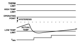
Figure 72. Increasing T<sub>MIN</sub> for Quieter Operation
