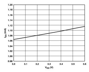
Figure 7. Normal I<sub>DD</sub> vs. Power Supply
