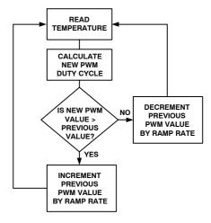
Figure 76. Enhanced Acoustics Algorithm
