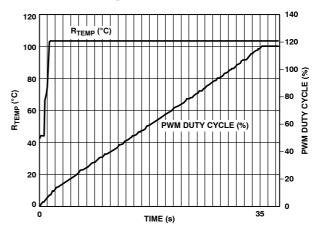
Figure 80. Enhanced Acoustics Mode with Ramp Rate = 1
