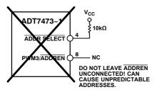
CARE SHOULD BE TAKEN TO ENSURE THAT PIN 8 (PWM3/ADDREN) IS EITHER TIED HIGH OR LOW. LEAVING PIN 8 FLOATING COULD CAUSE THE ADT7473-1 TO POWER UP WITH AN UNEXPECTED ADDRESS.
