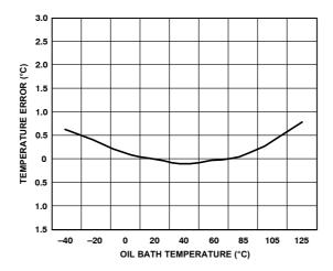
Figure 11. Remote Temperature Error vs. Temperature
