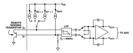
Figure 24. Signal Conditioning for Remote Diode Temperature Sensors
