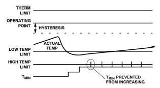
Figure 73. T<sub>MIN</sub> Adjustments Limited by the High Temperature Limit
