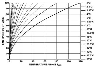
Figure 59. T<sub>RANGE</sub> vs. Actual Fan Speed Profile
