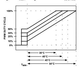
Figure 58. Increasing PWM $_{MIN}$  Changes Effective  $T_{RANGE}$
