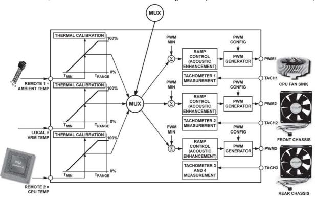
Figure 50. Assigning Temperature Channels to Fan Channels
