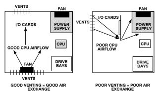
Figure 64. Chassis Airflow Issues
