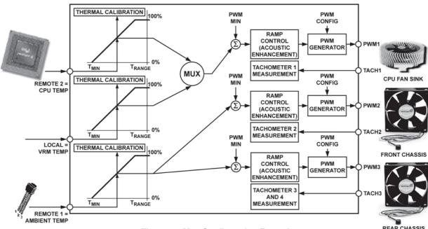
Figure 51. Mux Configuration Example
