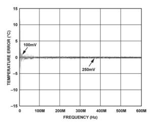
Figure 8. Internal Temperature Error vs. Frequency
