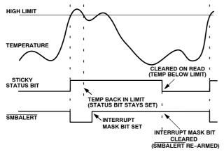
Figure 30. How Masking the Interrupt Source Affects
