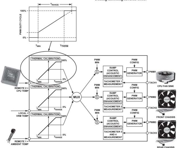
Figure 62. How T<sub>THERM</sub>Relates to Automatic Fan Control
