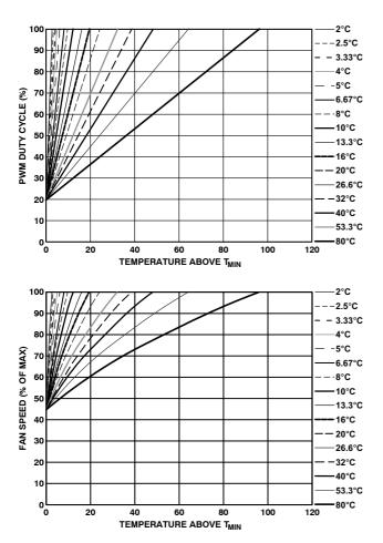
Figure 60. T<sub>RANGE</sub> and % Fan Speed Slopes with PWM<sub>MIN</sub> = 20%
