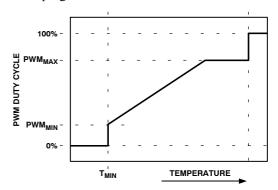
Figure 55. PWM<sub>MAX</sub> Determines Maximum PWM Duty Cycle Below the THERM Temperature Limit
