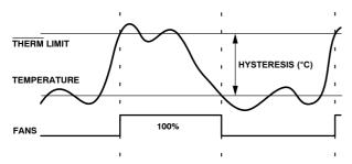
Figure 28. THERM Limit Operation
