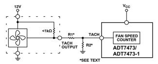
Figure 43. Fan with Strong TACH pullup to > V<sub>CC</sub> or Totem-Pole Output, Attenuated with R1/R2
