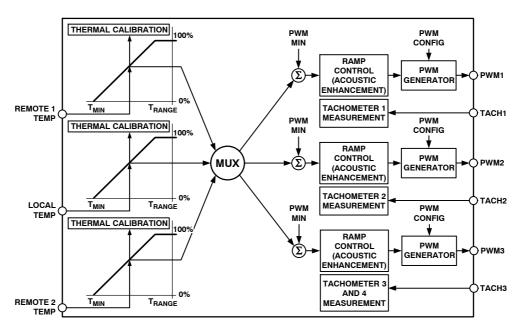
Figure 47. Automatic Fan Control Block Diagram
