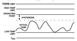
Figure 70. Temperature Between Operating Point and Low Temperature Limit
