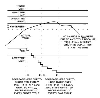
Figure 71. Effect of Exceeding Operating Point Minus
