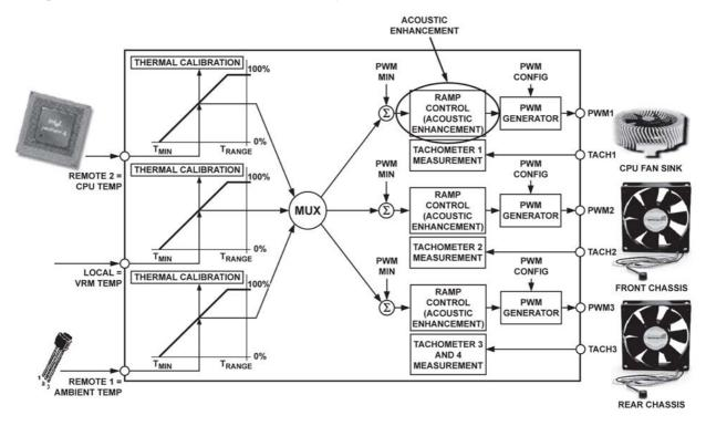
Figure 74. Acoustic Enhancement Smoothes Fan Speed Variations Under Automatic Fan Speed Control
