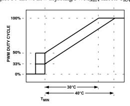
Figure 57. Adjusting  $PWM_{MIN}$  Affects  $T_{RANGE}$
