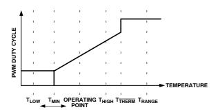
Figure 66. Dynamic T<sub>MIN</sub> Control Loop
