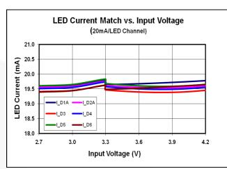
Figure 5. LED Current Match for all Six LED Channels at I<sub>LED</sub>=20mA
