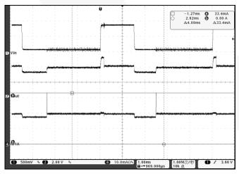
Figure 14. Line Transient from 1x to 1.5x Mode,  $V_{IN}$ =3.2V – 4.1V,  $I_{LEDx}$ =20mA
