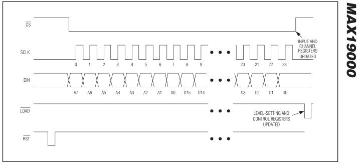
Figure 6. Serial-Port Timing with Asynchronous Load
