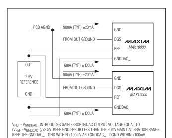
Figure 10. Sample Connection Diagram for Two Parts per Board
