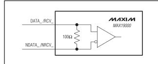
Figure 11. DATA\_ and RCV\_ Terminations
