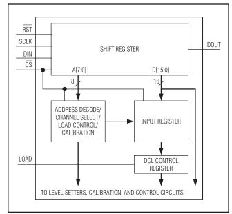
Figure 5. Serial-Interface Block Diagram
