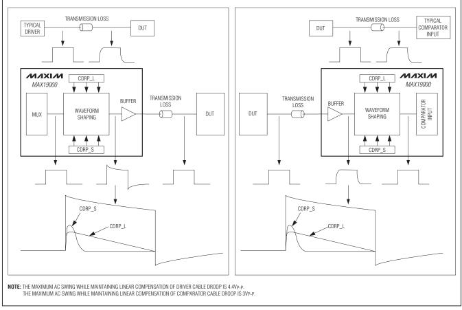
Figure 2. Driver/Comparator Cable-Droop Compensation
