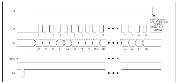
Figure 7. Serial-Port Timing with Synchronous Load (LOAD Held Low)
