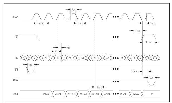
Figure 8. Detailed Serial-Port Timing Diagram
