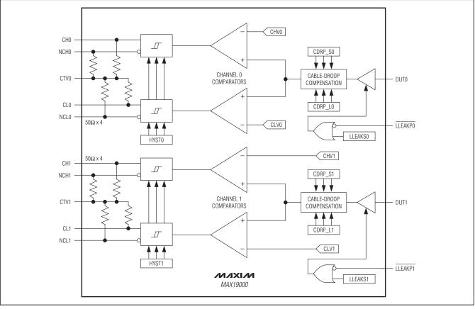
Figure 3. High-Speed Comparators Block Diagram
