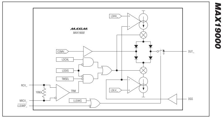
Figure 4. Active Load Block Diagram (One Channel Shown)
