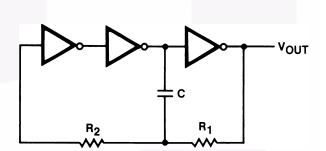
Figure 2. Stable RC Oscillator
