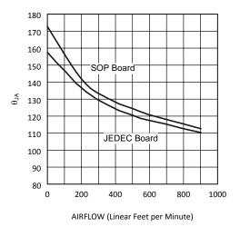
Figure 14.  $\theta_{JA}$  vs Airflow (SOIC-8)
