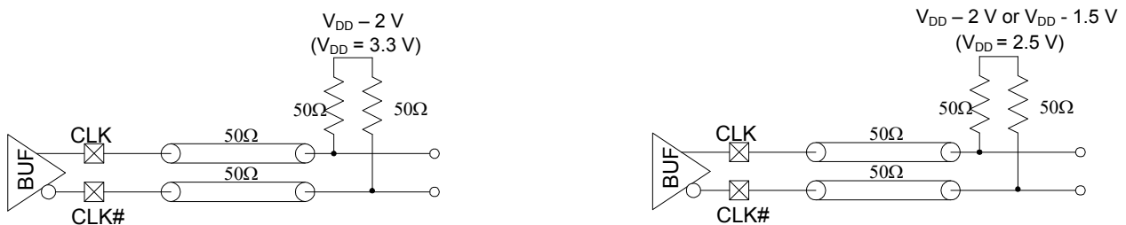
Figure 9. LVPECL Termination
