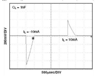
FIGURE 12. LOAD TRANSIENT RESPONSE
