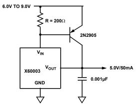
FIGURE 35. PRECISION 5V, 50mA REFERENCE
