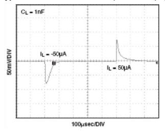
FIGURE 11. LOAD TRANSIENT RESPONSE
