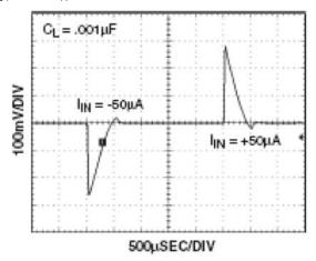
FIGURE 23. 50µA LOAD TRANSIENT RESPONSE
