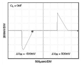
FIGURE 7. LINE TRANSIENT RESPONSE, NO CAPACITIVE LOAD
