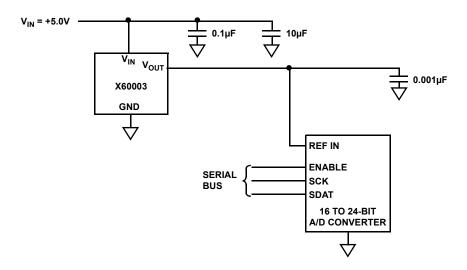
FIGURE 1. TYPICAL APPLICATION PRECISION 16 TO 24-BIT A/D CONVERTER
