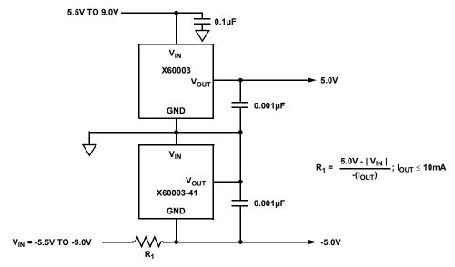
FIGURE 36. ±5.0V DUAL OUTPUT, HIGH ACCURACY REFERENCE
