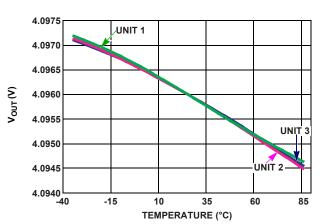
FIGURE 4. VOUT vs TEMPERATURE NORMALIZED TO +25°C (3 UNITS)
