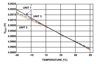
FIGURE 20.  $V_{OUT}$  vs TEMPERATURE (3 UNITS)
