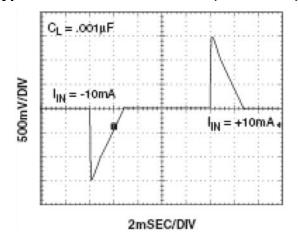
FIGURE 22. 10mA LOAD TRANSIENT RESPONSE
