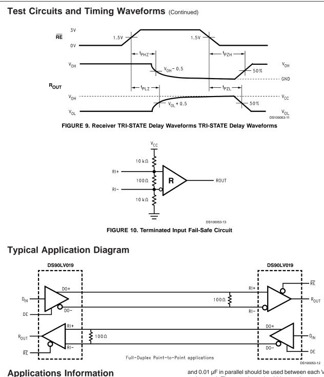
The DS90LV019 has two control pins, which allows the device to operate as a driver, a receiver or both driver and a receiver at the same time. There are a few common practices which should be implied when designing PCB for LVDS signaling. Recommended practices are:
