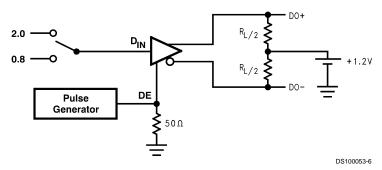
FIGURE 4. Driver TRI-STATE Delay Test Circuit
