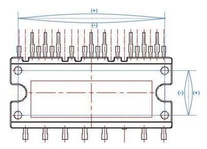
Figure 8. Flatness Measurement Position
