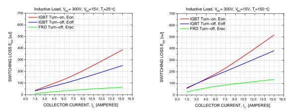
Figure 5. Switching Loss Characteristics
