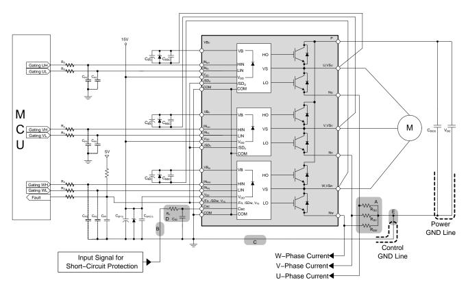
Figure 16. Typical Application Circuit
