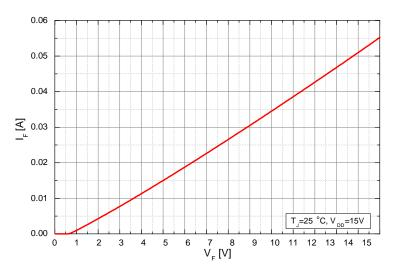
Figure 7. Built-In Bootstrap Diode Characteristics
