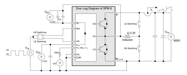
Figure 4. Example Circuit for Switching Test
