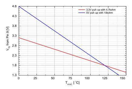
Figure 6. V-T Curve of Temperature Output of IC
