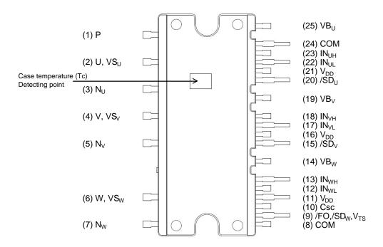
Figure 1. Pin Configuration – Top View
