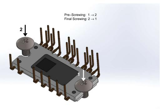
Figure 9. Mounting Screws Torque Order
