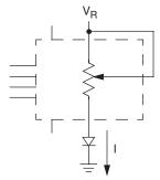
Two terminal variable resistor; variable current
