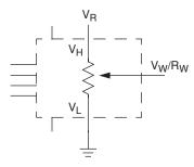
Three terminal potentiometer; variable voltage divider
