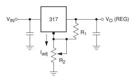
$V_O (REG) = 1.25V (1+R_2/R_1)+ladj R_2$
