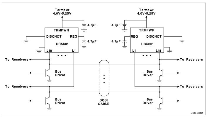
Typical SCSI Bus Configuration Using the UC5601
