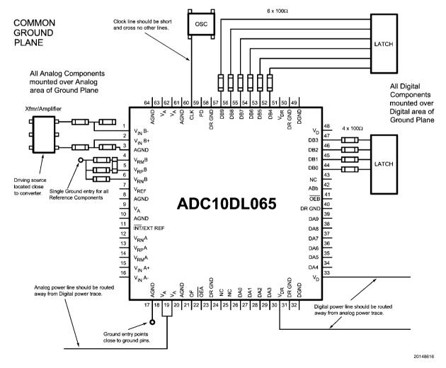
FIGURE 7. Example of a Suitable Layout
