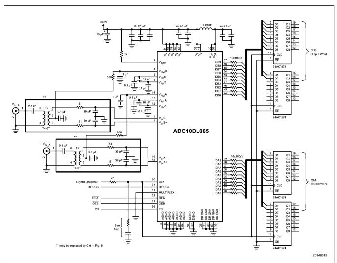
FIGURE 4. Application Circuit Using Transformer Drive Circuit, Parallel Mode
