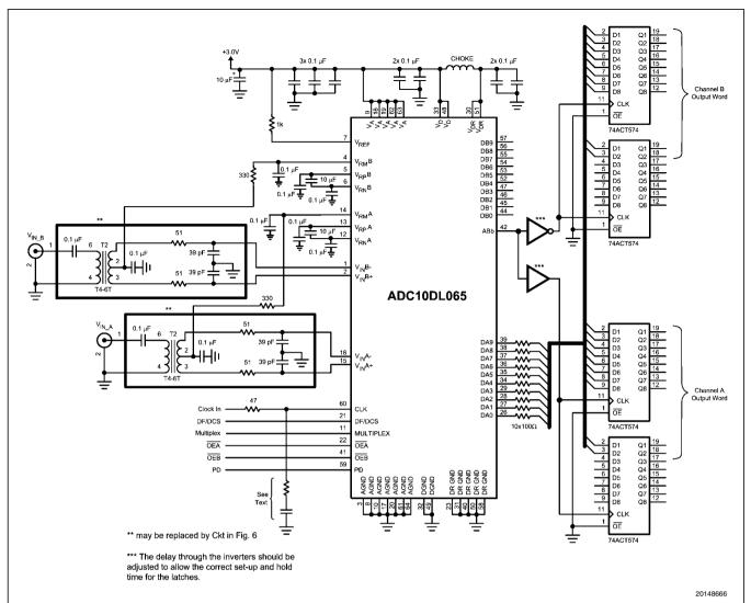
FIGURE 5. Application Circuit Using Transformer Drive Circuit, Multiplex Mode
