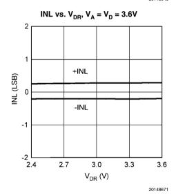
**Typical Performance Characteristics** Unless otherwise specified, the following specifications apply for AGND = DGND = DR GND = 0V,  $V_A = V_D = +3.3V$ ,  $V_{DR} = +2.5V$ , PD = 0V,  $V_{REF} = +1.0V$ ,  $f_{CLK} = 65$  MHz,  $f_{IN} = 32$  MHz,  $C_L = 15$  pF/pin, Duty Cycle Stabilizer On, parallel output mode. **Boldface limits apply for T**<sub>J</sub> = T<sub>MIN</sub> **to T**<sub>MAX</sub>: all other limits T<sub>J</sub> = 25°C
