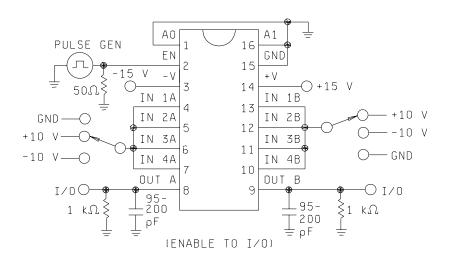
FIGURE 4. Switching times test circuits - continued.
