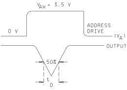
FIGURE 3. Break-before-make test circuit and waveforms – continued.
