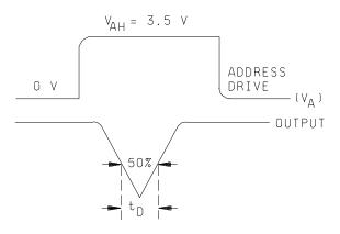
FIGURE 3. Break-before-make test circuit and waveforms – continued.
