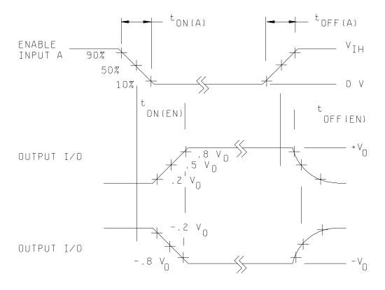
INPUT PULSE REQUIREMENTS  $V_{GEN} = 3 V_{thl(1)} = t_{thl(1)} \le 20 \text{ ns}$
