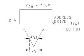
FIGURE 3. Break-before-make test circuit and waveforms.
