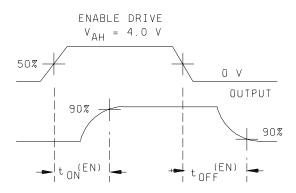
FIGURE 4. <u>Switching times test circuits</u> – continued.
