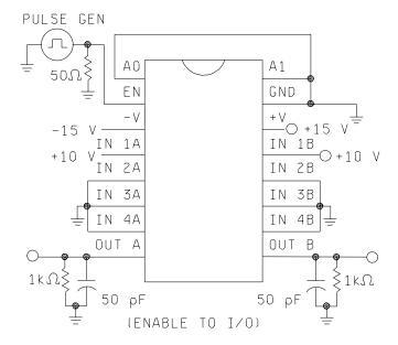
ENABLE DRIVE  $V_{\rm AH} = 4.0~{\rm V}$  for device type 03
