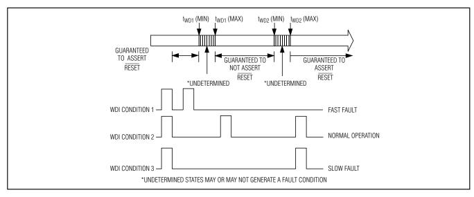
Figure 1. MAX6752/MAX6753 Detailed Watchdog Input Timing Relationship
