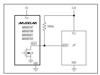
Figure 6. Interfacing to Other Voltage Levels
