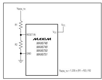
Figure 2. Calculating the Monitored Threshold Voltage (VMON\_TH)
