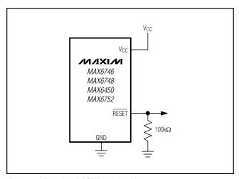
Figure 7. Ensuring RESET Valid to V<sub>CC</sub> = 0
