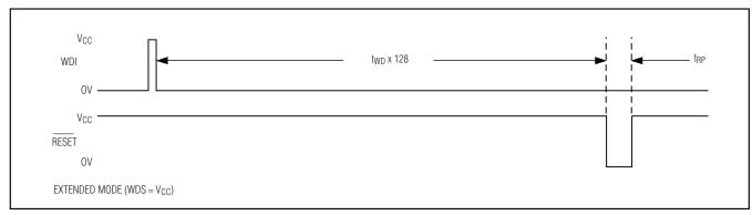
Figure 4b. Watchdog Timing Diagram, WDS = VCC
