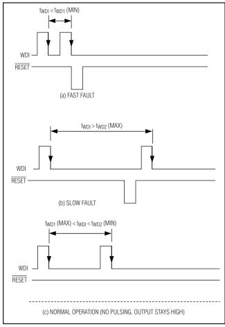
Figure 5. MAX6752/MAX6753 Window Watchdog Diagram
