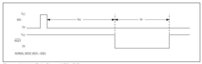
Figure 4a. Watchdog Timing Diagram, WDS = GND
