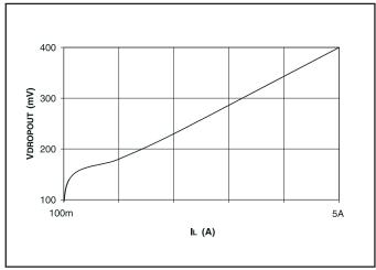
Figure 2. Typical dropout (VIN - VOUT), TJ = 27°C.
