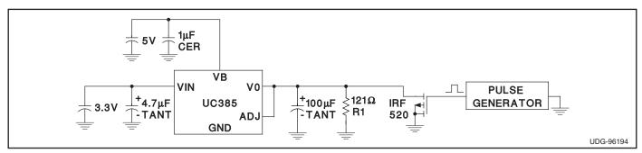
Figure 6. Transient test circuit.
