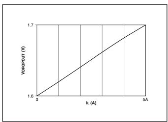
Figure 1. Typical dropout (VB - VOUT), TJ = 27°C.
