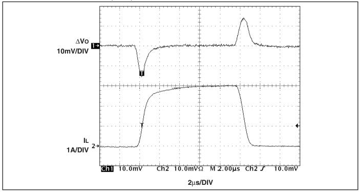
Figure 7. 10mA to 3A/µs load transient response.
