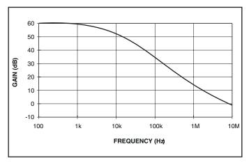
Figure 4. Open loop gain (100μf output capacitance, 1A load).
