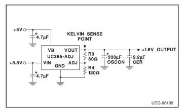
Figure 8. Typical UC385-ADJ application.
