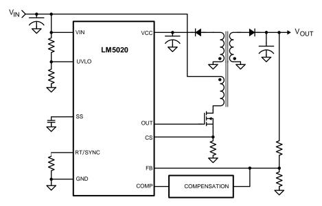
Figure 1. Non-Isolated Flyback Converter
