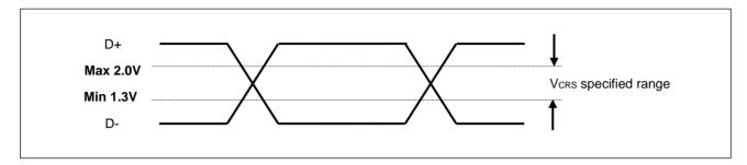
5. They indicate rising time (Trise) and falling time (Tfall) of the full-speed differential data signal. They are defined by the time between 10% and 90% of the output signal voltage. For full-speed buffer, Tr/Tf ratio is regulated as within ±10% to minimize RFI emission.
