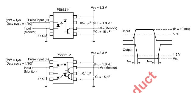
Remark CL is approximately 15 pF which includes probe and stray wiring capacitance.
