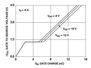
Figure 7. Gate Charge Characteristics
