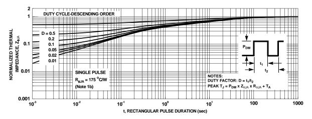
Figure 12. Junction-to-Ambient Transient Thermal Response Curve
