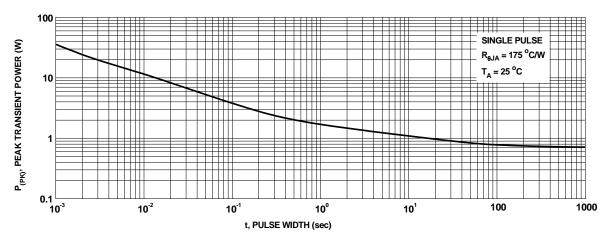
Figure 11. Single Pulse Maximum Power Dissipation
