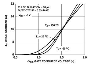
Figure 5. Transfer Characteristics
