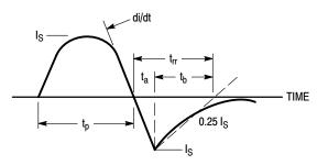
Figure 14. Diode Reverse Recovery Waveform
