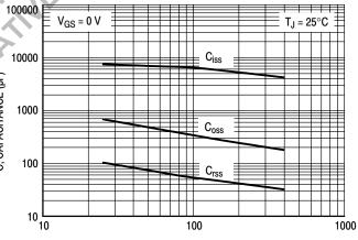
Figure 7b. High Voltage Capacitance Variation
