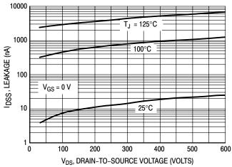
Figure 6. Drain-To-Source Leakage Current versus Voltage
