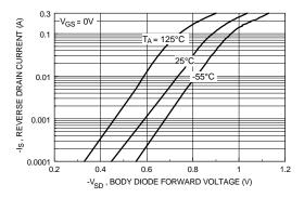
Figure 16. Body Diode Forward Voltage
