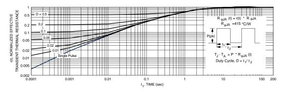
Figure 21. Transient Thermal Response Curve.
