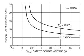
Figure 14. On-Resistance Variation with Gate-to-Source Voltage.
