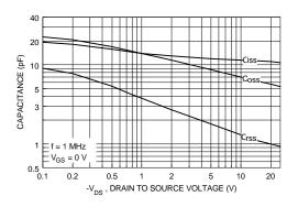
Figure 18. Capacitance Characteristics.
