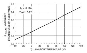
Figure 13. On-Resistance Variation with Temperature.
