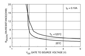
Figure 4. On-Resistance Variation with Gate-to-Source Voltage.
