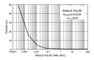
Figure 20. Single Pulse Maximum Power Dissipation.
