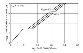
Figure 17. Gate Charge Characteristics.
