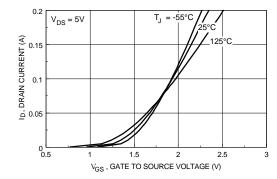
Figure 5. Transfer Characteristics.
