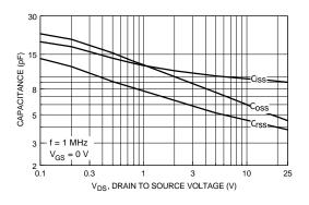
Figure 8. Capacitance Characteristics.
