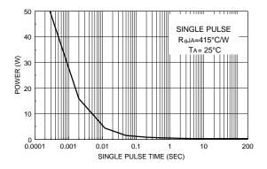
Figure 10. Single Pulse Maximum Power Dissipation.
