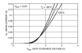
Figure 15. Transfer Characteristics.
