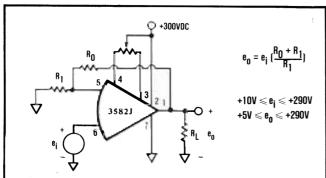
FIGURE 3. Operation from a Single Supply.
