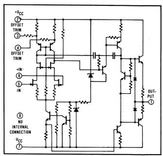
FIGURE 1. Simplifier Schematic of 3580
