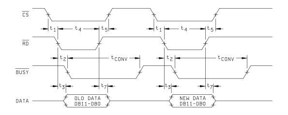
FIGURE 6. ROM mode, parallel read bus timing diagrams.
