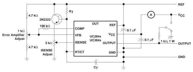
Figure 6. Open-Loop Laboratory Test Fixture
