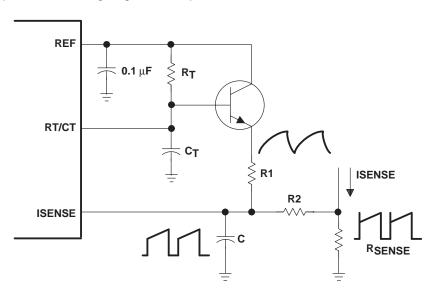
Figure 8. Slope Compensation
